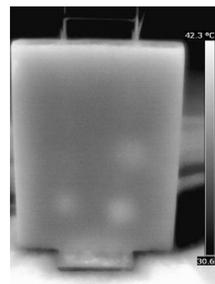
Fig. 7. Infrared picture of the slab : passive thermography (the only source of heating is the sun)
